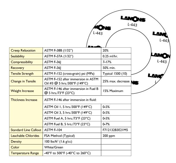
A compressed sheet gasket material utilizing a neoprene binder. This material has an inherent resistance to oil and petroleum based solvents.
