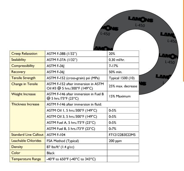
A compressed gasket material with a reinforcement structure consisting of glass and aramid fibers. Excellent resistance to steam can be realized due to the addition of glass fiber. A premium nitrile binder is utilized to achieve resilience and additional chemical resistance.
